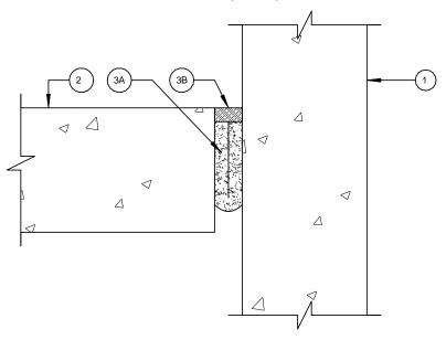
1. **Wall Assembly** – Min 4 1/2 in. (114 mm) thick reinforced lightweight or normal weight (100 – 150 pcf or 1600-2400 kg/m³) structural concrete. Wall may also be constructed of ant UL Classified **Concrete Blocks\*.**
