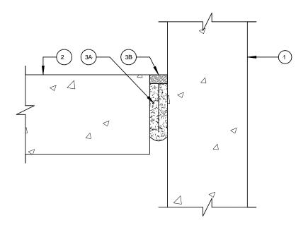
1. **Wall Assembly** – Min 4 1/2 in. (114 mm) thick reinforced lightweight or normal weight (100 – 150 pcf or 1600-2400 kg/m³) structural concrete. Wall may also be constructed of ant UL Classified **Concrete Blocks\*.**
