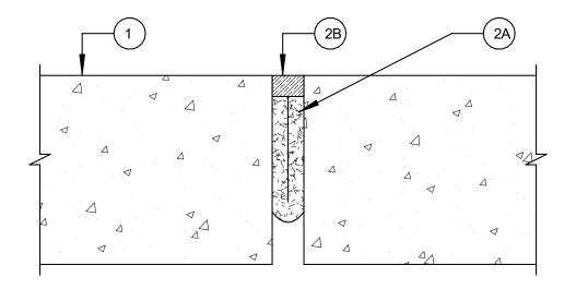
1. **Wall Assembly** – Min 4 ½ in. thick reinforced lightweight or normal weight (100 – 150 pcf) structural concrete. Wall may also be constructed of any UL Classified **Concrete Blocks**\*.
