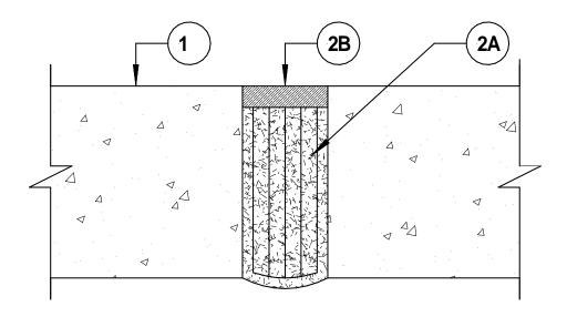
1. **Wall Assembly** – Min 4 ½ in. thick reinforced lightweight or normal weight (100 – 150 pcf) structural concrete. Wall may also be constructed of any UL Classified **Concrete Blocks\***.
