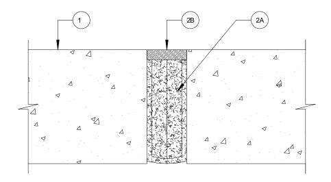
1. **Wall Assembly** – Min 5-3/4 in. (146 mm) thick reinforced lightweight or normal weight (100 – 150 pcf or 1600-2400 kg/m³) structural concrete. Wall may also be constructed of any UL Classified **Concrete Blocks**\*.
