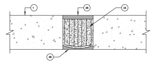
1. **Wall Assembly** – Min 4 ½ in. (114 mm) thick reinforced lightweight or normal weight (100 – 150 pcf or 1600-2400 kg/m³) structural concrete. Wall may also be constructed of any UL Classified **Concrete Blocks**\*.
