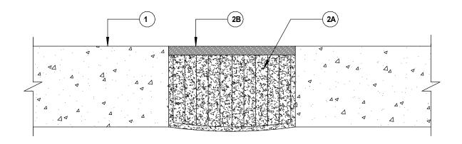
1. **Wall Assembly** – Min 4 ½ in. thick reinforced lightweight or normal weight (100 – 150 pcf) structural concrete. Wall may also be constructed of any UL Classified Concrete Blocks\*.
